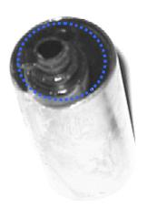
3, Test fit the piston with the cylinder. When you move the piston inside the cylinder you should feel a certain level of resistance. If there is no resistance at all, the piston O'ring is no good (it is allowing too much air leakage, which can result in real serious performance drop). On the other hand, if there is too much resistance, the spring will have a hard time pushing the piston and will lead to Page 18 Copyright 2005,06 **The AirsoftPRESS (Hong Kong)**. All rights reserved.
