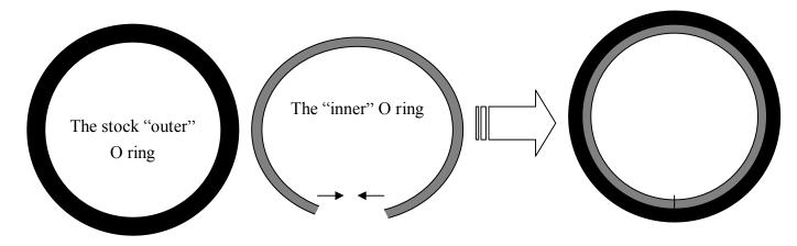
Put it in first, then put your stock O ring back in (so your stock O ring can wrap around the thinner O ring). This way you can slightly increase the effective dimension of the "outer" O ring (for better compression) and at the same time retain some "flexibilities" without introducing too much friction along piston movement (an oversized O ring can produce too much friction and lead to fast wear and tear on the O ring rubber as well as serious FPS drop).
