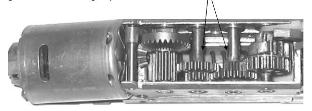
If you are replacing some or all of the stock gears with third party gears, always try to mesh the gears by hand and see if they fit together well. In fact it is always suggested that you buy all four gears from the same manufacturer to ensure the best possible fitting.
