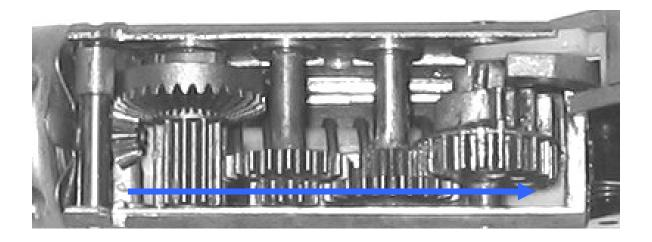
Be careful when shimming the bevel gear. You must ensure that the anti-reversal latch can maintain proper alignment with it. This issue is often ignored by beginners – a latch with improper alignment can damage or wear out real fast.
