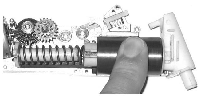
Our **Practical AEG Upgrade** guide covers in-depth the issue of spring, spring guide and piston fitting.
