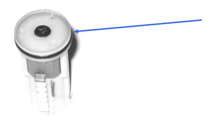
You may also apply grease around the cylinder head for better air sealing. Since the cylinder head does not move, in theory its O ring should not wear out by itself. Still, you may want to regularly check and reapply grease around it if necessary during your regular maintenance effort.
