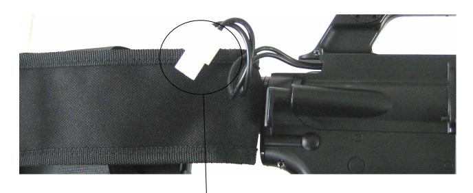
Large Tamiya battery plug. We use it only because most standard size battery packs use this type of plug. You may stick with the stock small plug if you wish as it doesn't really hurt (at the power level of most A15 configurations) anyway.
