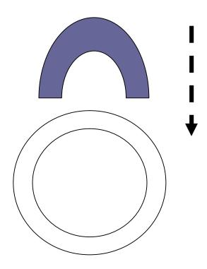
The "cut" in the middle is produced by pressing down the arc shaped spacer onto the hop up rubber. If for some reasons the two ends of the spacer are not evenly worn out (or if one end breaks while the other one remains intact), unexpected spinning effect will be produced. Regularly perform visual check (by looking through the barrel) to ensure that the spacer is in good shape.
