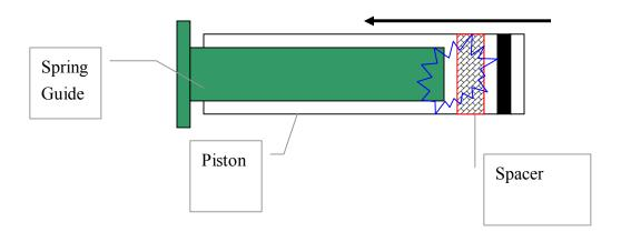
We found that using spacer for better FPS is effective and safe only for harder and shorter springs. On soft and long springs the small increase in FPS has no real world significance at all.
