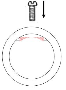
This is a trial and error process. If the rubber is pressed down too much, your bullets will fly to the 3<sup>rd</sup> floor. Adjust the screw little by little until the desired range is achieved.
