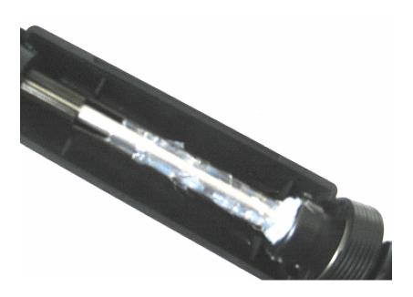
No worry, the glue can be easily removed with a screw driver.
