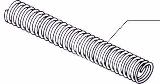
If a stock TM spring is rated at 100%, the A-15 stock spring is at the most 85%.
