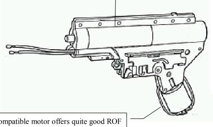
The EG-560 compatible motor is attached to the mechbox via 2 screws. These screws will get loose after several thousand rounds of firing.
