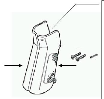
The two halves of the plastic hand grip are affixed together and attached to the receiver through several small screws. Holding the hand grip effectively puts the entire weight load of the gun onto the screws. Not reinforced in any way, this structure is highly fragile.
