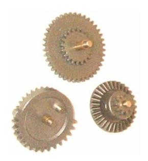
The goal of shimming is to keep the spacing of gears correct. Most shim washers in the market have sizes of 0.2mm, 0.3mm and 0.5mm. There are 0.15mm and 0.1mm available from some Japanese manufacturers too. Use the SMALLEST possible shim washers to make the finest possible adjustment.
